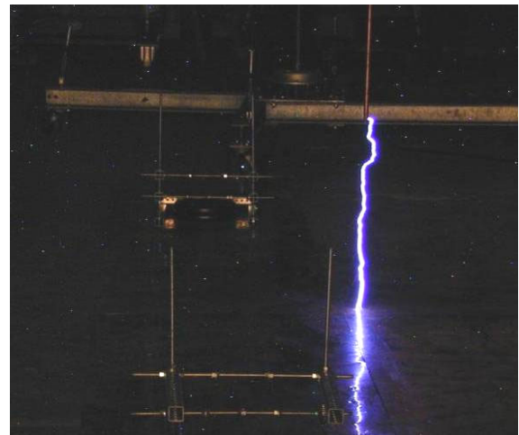
(d) Flash to the ground, positive polarity H = 73 \text{ cm} , h_g = 24.3 \text{ cm} , X = 48.2 \text{ cm}
