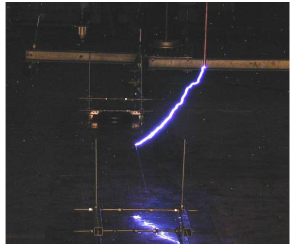
(b) Flash to the line, positive polarity H = 73 \text{ cm} , h_g = 24.3 \text{ cm} , X = 48.2 \text{ cm}
