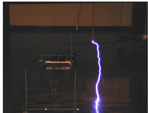
(d) Flash to the ground, positive polarity H = 73 \text{ cm} , h_t = 23.5 \text{ cm} , X = 45 \text{ cm}
