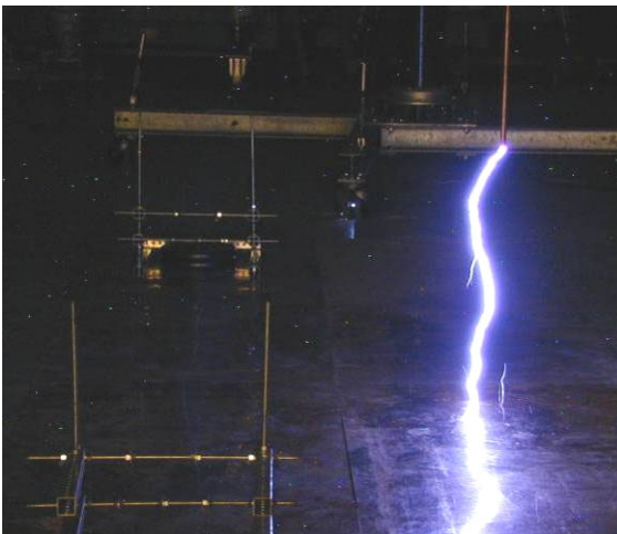
(c) Flash to the ground, negative polarity H = 73 \text{ cm} , h_g = 24.3 \text{ cm} , X = 87.7 \text{ cm}
